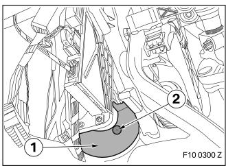
Connect branch **A1** on retrofit wiring harness **A** to emergency power siren **D**.
