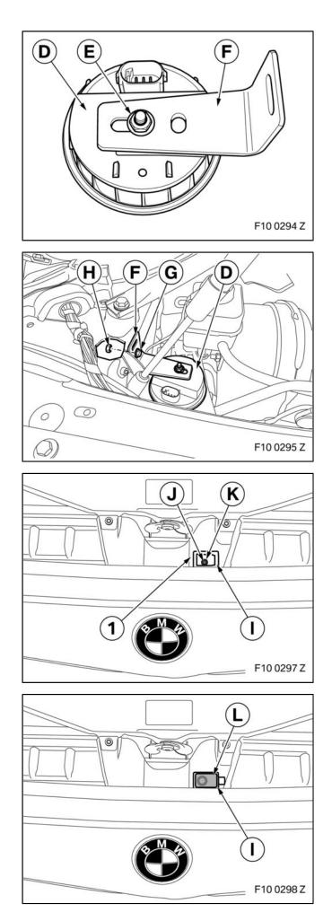
Secure emergency power siren **D** using hexagon nut **E** to emergency power siren holder **F**.
