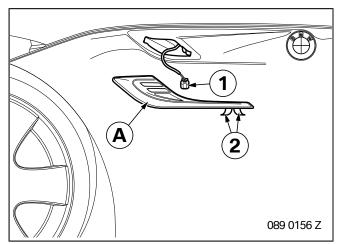
Break off aligning pin (1) flush with additional turn indicator (2).
