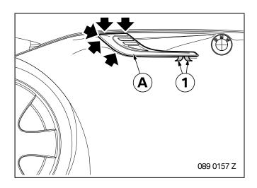
Align additional turn indicator **A** flush with the contour of the side panel.
