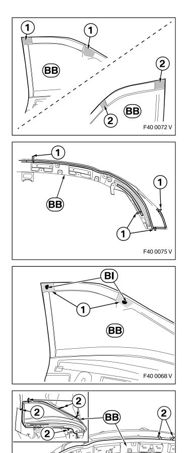
Abrade and clean the areas (1) on the **inside** and the areas (2) on the **outside** of the underbody console **BB** using suitable materials.
