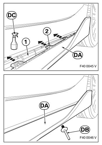
Cut the expanding rivets on the standard side sill insert using suitable tools and remove the standard side sill insert, starting from the front.
