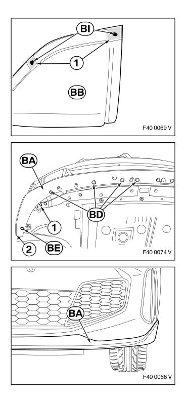
Apply a dot of liquid adhesive **BI** on the outside of the underbody console **BB** in each of the marked areas (1).
