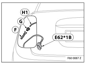
Disconnect, insulate and tie back the BROWN cable from PIN 5 on the left rear light plug **E62\*1B**.
