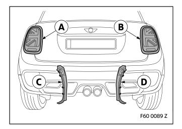
Install rear lights **A** and **B** with left gutter cover **C** and right gutter cover **D** as described in **ISTA/AIR 63 12 275**.
