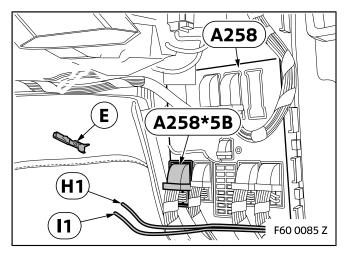
Crimp socket contacts **E** to branch **H1**, BLUE/YEL-LOW cable, and connect them to PIN 13 in plug **A258\*5B** on the BDC **A258**.
