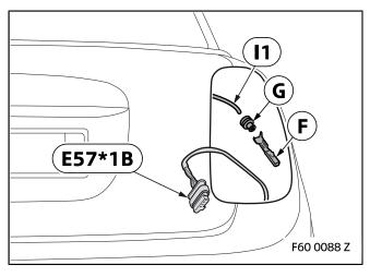
Disconnect, insulate and tie back the BROWN cable from PIN 5 on the right rear light plug **E57\*1B**.
