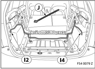
Route branches **I2** and **H2** along the right-hand side of the car and then further through the boot, as shown, and secure them with cable tie **J**.
