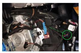
On the F25 steering wheels, just unplug the connector from the right switch unit so that you can take it out together with the clasp.
