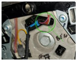
So that you can take out the entire switch unit with the cable set, you have to unplug it. The cable set from the steering wheel buttons and that from the airbag
