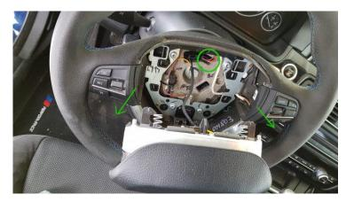
it out to the front. Hold the screwdriver as vertically as possible so that the lock is caught.
