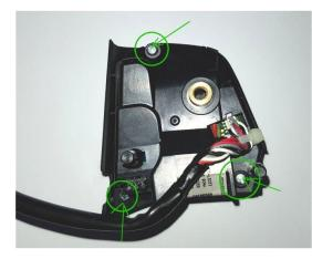
The button wheel with its holder is screwed inside again. Unscrew these two screws as well. Now you can take out the button wheel of its bracket. As with the right switch unit, there are 3 screws on the back, unscrew them to open the switch unit.
