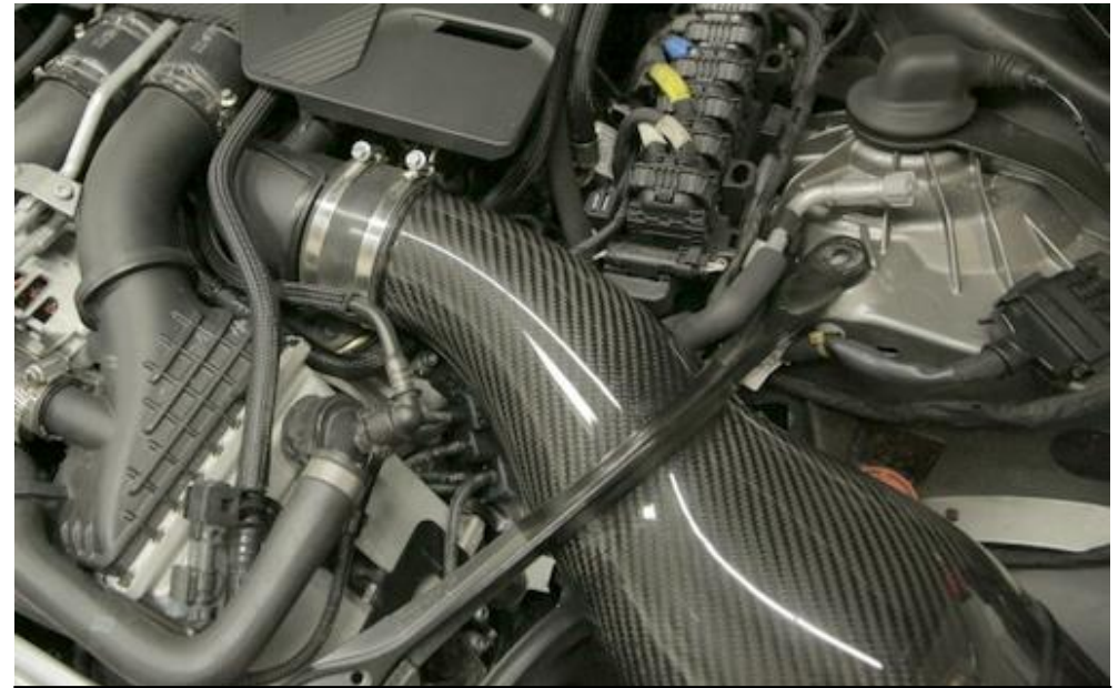
29. Now lower the rear of the housing into the silicon hose. Do not tighten yet.
