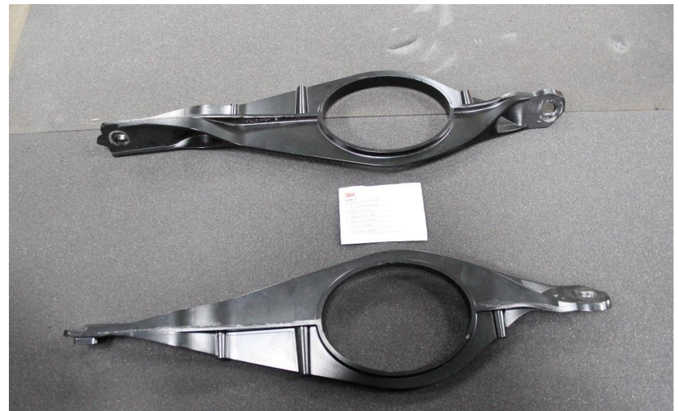
20. Take the strut braces and the cleaning wipe supplied – clean the inside surfaces of the oval openings.
