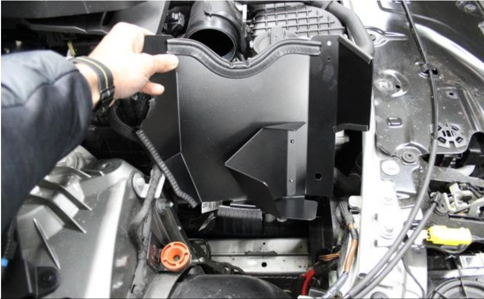
9. Starting from the Left side – lower the shield into the engine bay.
