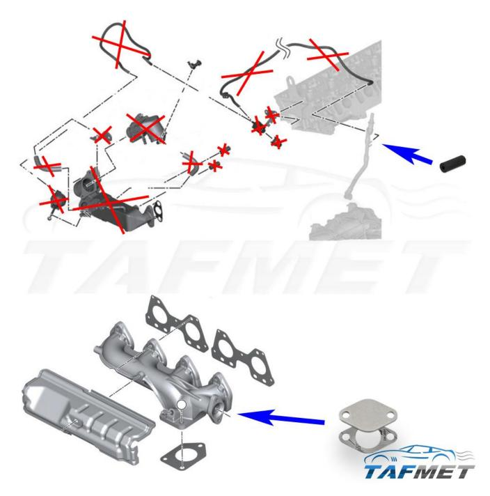
The exit from the exhaust manifold to the EGR system is blocked with a blanking plate with a gasket that are present in the kit.
