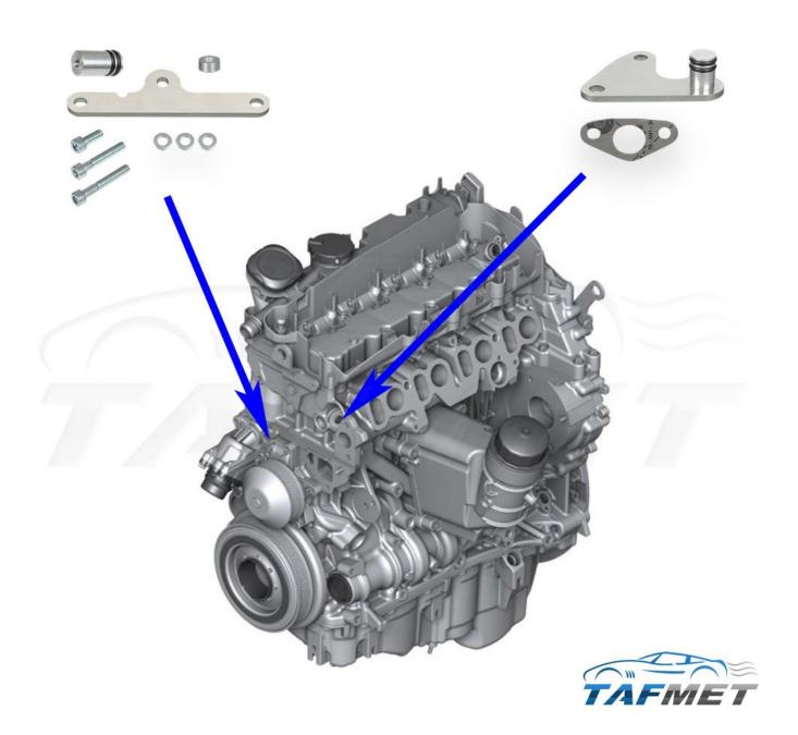
On the left and right side of the water pump, you need to use the longer bolt.
