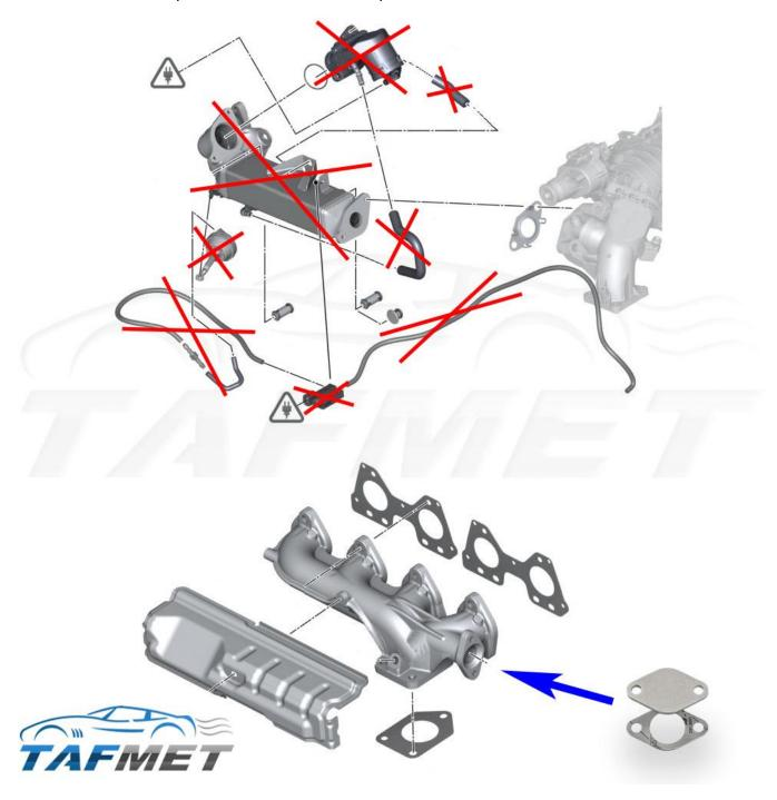
The exit from the exhaust manifold to the EGR system is blocked with a blanking plate with a gasket that are present in the kit.
