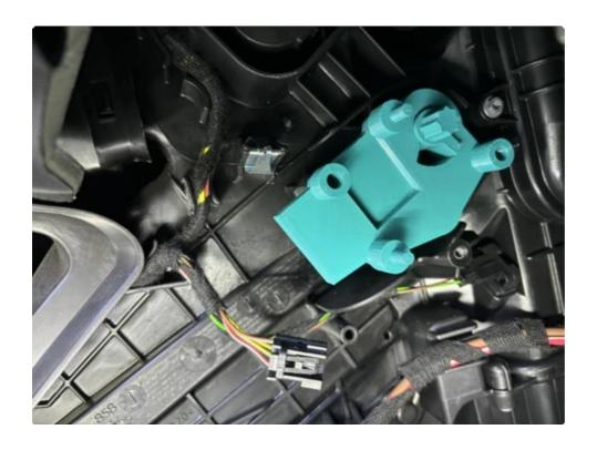
8. Install the actuator with the longer screws that is included in the kit.
