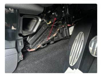
3. First removing the plug on the actuator (Car need to be off)
