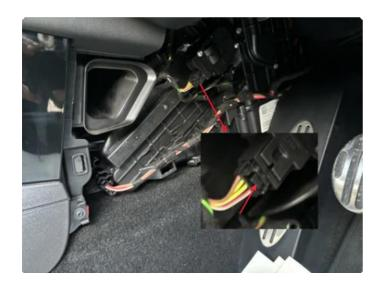
4. Second remove the two screws holding the actuator in palace.
